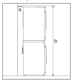
The Miele washing machine can be installed as part of a washer-dryer stack in combination with a Miele tumble dryer. An appropriate "stacking kit" is required (part # 12 996 026).
